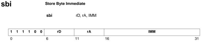
Stores the contents of the least significant byte of register rD, into the memory location that results from adding the contents of register rA and the value IMM, sign-extended to 32 bits.
